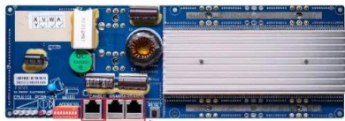
ESM5 * Communication between battery and server Band rate: 9600bps ESM5 Interface * Communication between parked packs or EMS and PC Band rate: 9600bps
