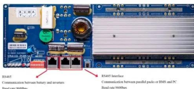
ES485 Communication between battery and server Band rate: 9600bps ES485 Interface Communication between parallel packs or EMS and PC Band rate: 9600bps
