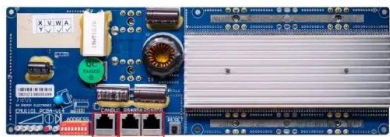
RS485 Communication between battery and inverter Baud rate:9600bps RS485 Interface Communication between parallel packs or BMS and PC Baud rate:9600bps
