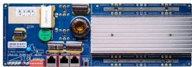
RS485 * Communication between battery and inverter Band rate: 100Kbps RS485 Interface * Communication between parallel packs or BMS and PC Band rate: 500Kbps
