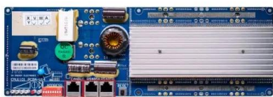
ES485 * Communication between battery and inverter Baud rate:9600bps ES483 Interface * Communication between parallel packs or BMS and PC Baud rate:9600bps
