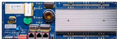
RS485 * Communication between battery and inverter Baud rate:9600bps RS485 interface * Communication between parallel packs or BMS and PC Baud rate:9600bps
