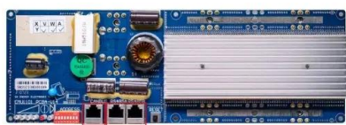
RS485 Communication between battery and inverter Board case:10000tp. RS485 Interface Communication between parallel packs or BMS and PC Board case:10000tp.
