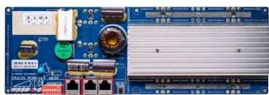
RS485 Communication between battery and inverters Board size: 9000kpc RS485 Interface Communication between parallel packs or BMS and PC Board size: 9000kpc
