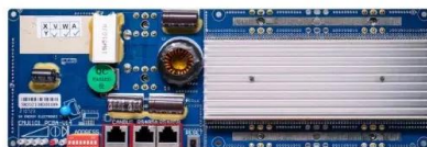
RS485 Communication between battery and inverter Baud rate: 9600bps RS485 interface Communication between panel/pack or BMS and PC Baud rate: 9600bps
